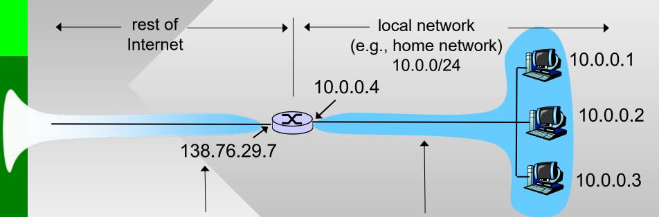
All datagrams *leaving* local network have the same single source NAT IP address: 138.76.29.7, different source port numbers Datagrams with source or destination in this network have 10.0.0/24 address for source, destination (as usual)
