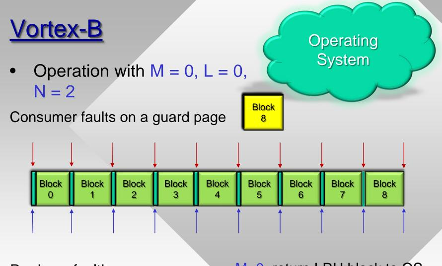
Producer fault! M=0, return LRU block to OS The producer installs a guard page and must wait for the consumer N=2
