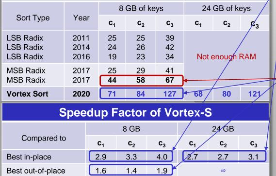
Vortex is 2.9-4.0x faster Vortex is 2.9-4.0x faster at sorting 8 GB than the at sorting 24 GB than nearest in-place radix the nearest in-place sort competitors radix sort competitors
