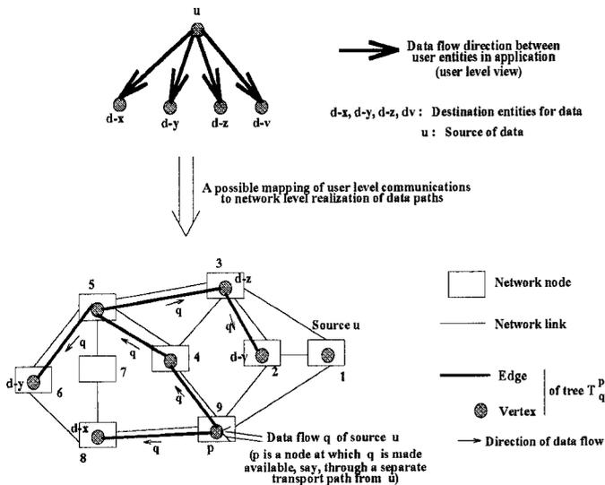
Figure 1: Tree-structured paths for multicasting
