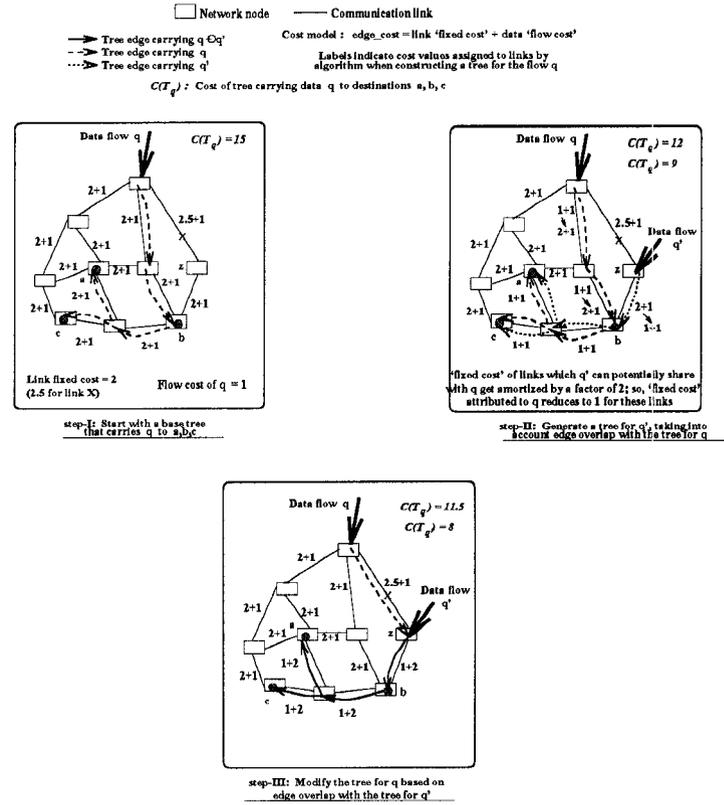
Figure 5: Tree setup scenario, with changing link costs
