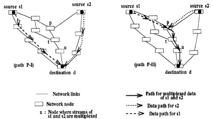
Figure 2: ‘path sharing’ to reduce transport cost
