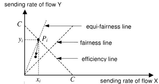
Fig. 2. Two-flow binary-feedback control system.
