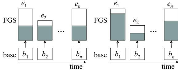
**Figure 1. Scaling of MPEG-4 FGS using fixed-size (left) and variable-size (right) frames.**
