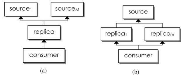
Fig. 1. System model (arrows signify the direction of information requests). (a) Aggregation. (b) Backup/load-balancing.
