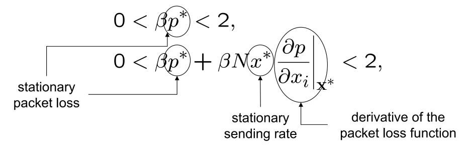
Stability conditions do not depend on any delays or the routing matrix of end-flows!
