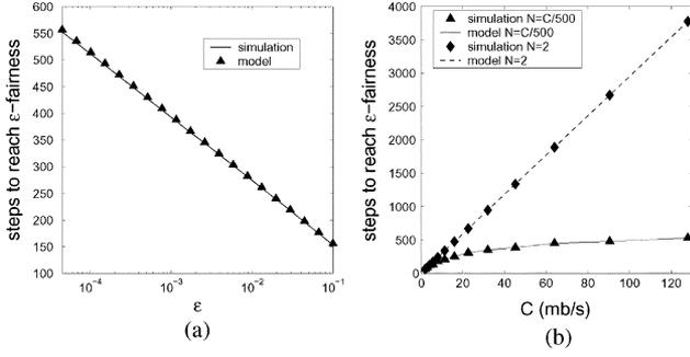
Fig. 3. (a) Verification of model (58) against EMKC simulations ( $C = 1$  mb/s,  $\alpha = 10$  kb/s, and  $\beta = 0.5$ ). (b) Exponential and linear rates of convergence to fairness for EMKC ( $\varepsilon = 0.1$ ).
