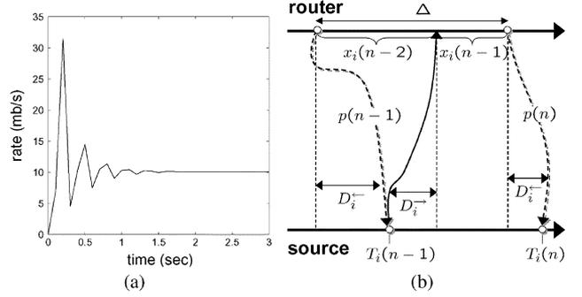
Fig. 6. Naive EMKC implementation: (a) one ns2 flow ( $\alpha = 100$  kb/s,  $\beta = 0.9$ , and  $\Delta = 50$  ms) passes through a bottleneck link of capacity 10 mb/s; (b) inconsistent feedback and reference rate.
