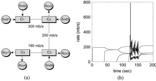
Fig. 9. (a) “Parking lot” topology; (b) Naive implementation of EMKC ( $\alpha = 10$  mb/s and  $\beta = 0.9$ ) in the “parking lot” topology.
