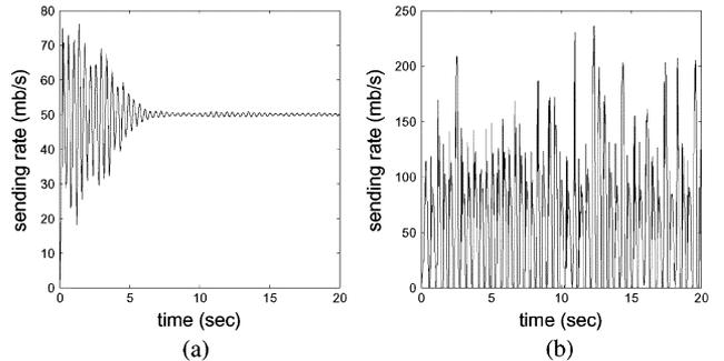
Fig. 2. Simulation results of the classic Kelly control under different delays ( $\kappa = 1/2$ ,  $\omega = 20$  kb/s,  $C = 50$  mb/s). (a)  $D = 90$  ms and (b)  $D = 120$ .
