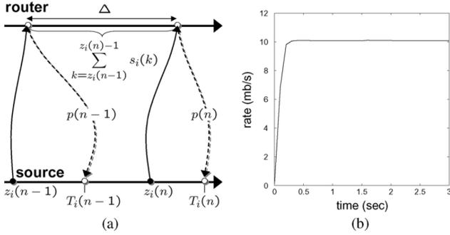
Fig. 7. Proper EMKC implementation: (a) graphical explanation of the algorithm; (b) one ns2 flow ( $\alpha = 100$  kb/s,  $\beta = 0.9$ , and  $\Delta = 50$  ms) passes through a link of capacity 10 mb/s.
