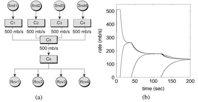
Fig. 8. Four EMKC ( $\alpha = 10$  mb/s,  $\beta = 0.9$ , and  $\Delta = 100$  ms) flows in the “dumb bell” topology.
