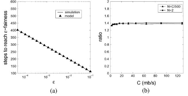
Fig. 4. (a) Verification of model (65) against AIMD simulations ( $C = 1$  mb/s,  $\alpha = 10$  kb/s, and  $\beta = 0.5$ ). (b) Ratio  $\theta_M/\theta_A$  for fixed and variable  $N$ .
