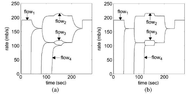
Fig. 10. Proper implementation of EMKC ( $\alpha = 10$  mb/s,  $\beta = 0.9$ , and  $\delta = 0.01$ ) in the “parking lot” topology. (a) Constant delay; (b) random delay.
