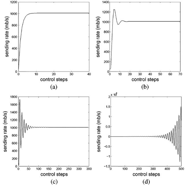
Fig. 1. Stability of Kelly control under different feedback delays ( $\kappa = 1/2$ ,  $\omega = 10$  mb/s, and  $C = 1000$  mb/s). (a)  $D = 1$ , (b)  $D = 2$ , (c)  $D = 3$ , and (d)  $D = 4$ .
